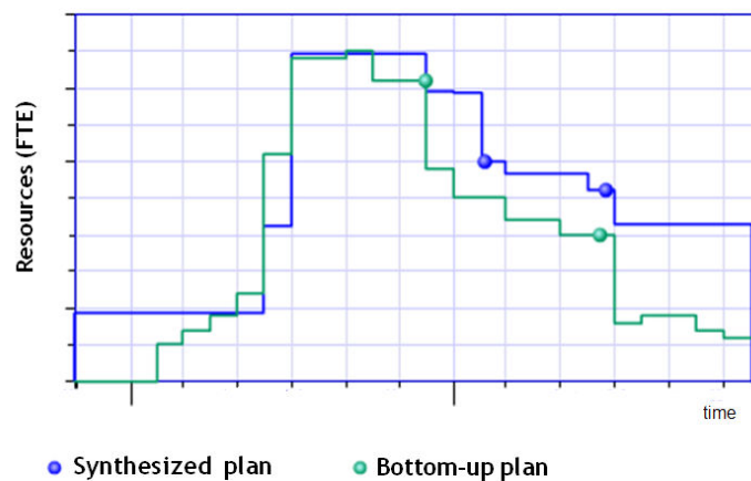
Figure 3: The ability to very quickly create a top-down synthesized plan that then drives the manager's bottom-up plan enables managers to readily observe potential areas of resource shortage and eventually reconcile the two plans.
